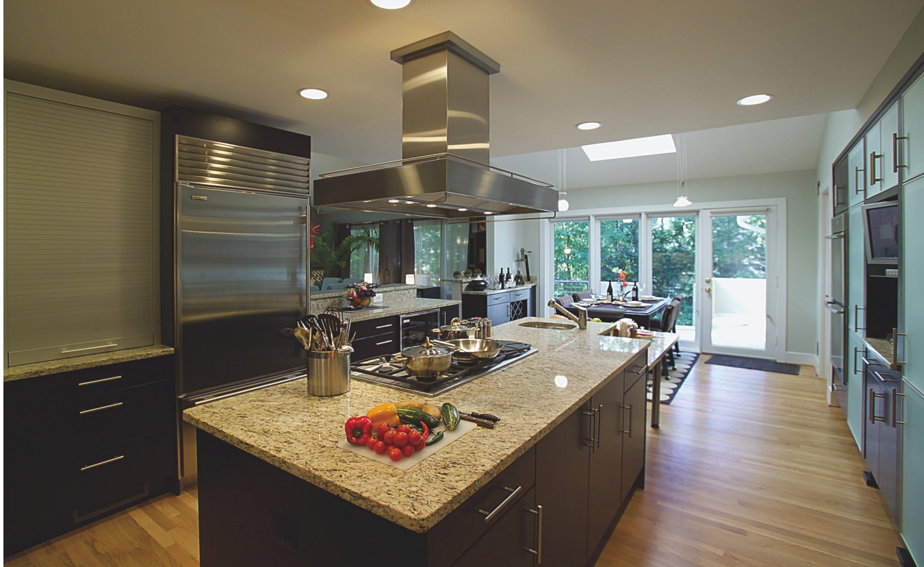
The existing range hood was replaced with a sleek stainless steel version above the new island. Although the hood had to be relocated slightly, the remodeler was able to tie it into the existing vent ductwork that ran through the attic space directly above it.
